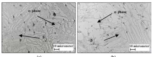
(a) (b) **Figure 2.** Microstructure of titanium alloy sintered implants (a) implant A, and (b) implant B.
